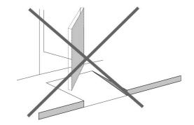
Exposed corners must be rounded or in bevelled angle to avoid becoming hazardous. Platform edges must be clearly highlighted.
