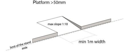
Level landings must be provided at the top and the bottom of the ramp and at every intermediate level where an exit door can be opened.
